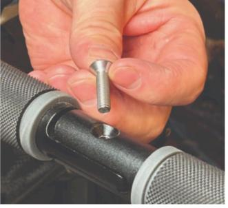
Al. Locate the screw at the center folding hinge of the U-shaped grip bar of the Veloped. Unscrew the screw with the included 4mm allen key and remove it.
