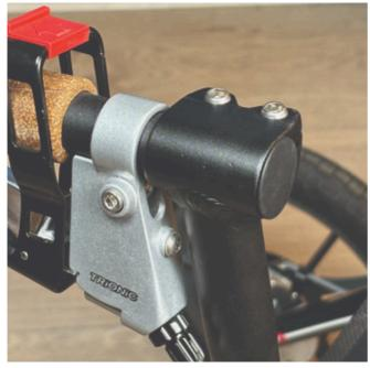
Al. On top of the black semi-vertical tube, locate the two screws that clamp the grip tube, situated in front of the brake lever.
