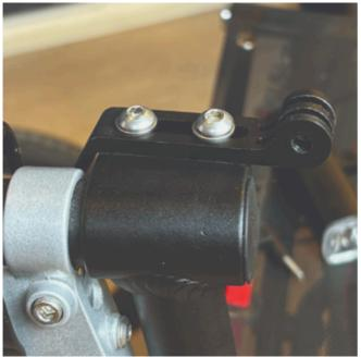
**A6.** Identify the circular front end of the light holder, with two slots for attaching the light.
